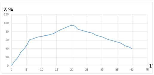
Figure-2. Protection level as a function of temperature.
